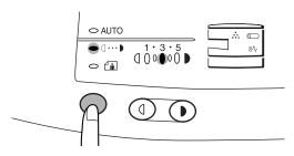
Press and hold down the exposure mode selector key for approximately 5 seconds. The manual (4···•) indicator will go out and the photo (1) indicator will begin to blink. The exposure indicator marked "5" will light up, indicating the standard toner mode is active.
